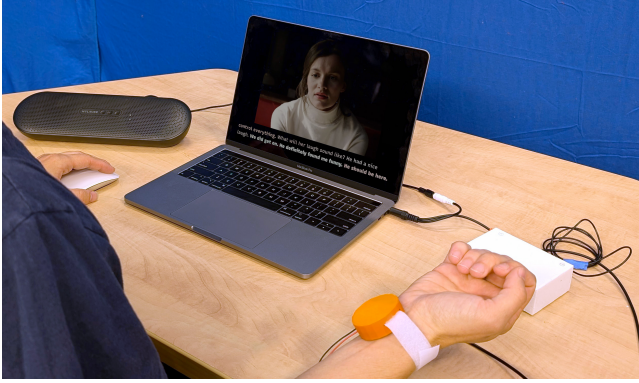
Figure 2: To watch videos, participants would strap the voice coil to their arm, with the device face-down against the inside of their wrist. A laptop would drive both the haptic signals and an external speaker, that played the original sounds coming from the videos.
